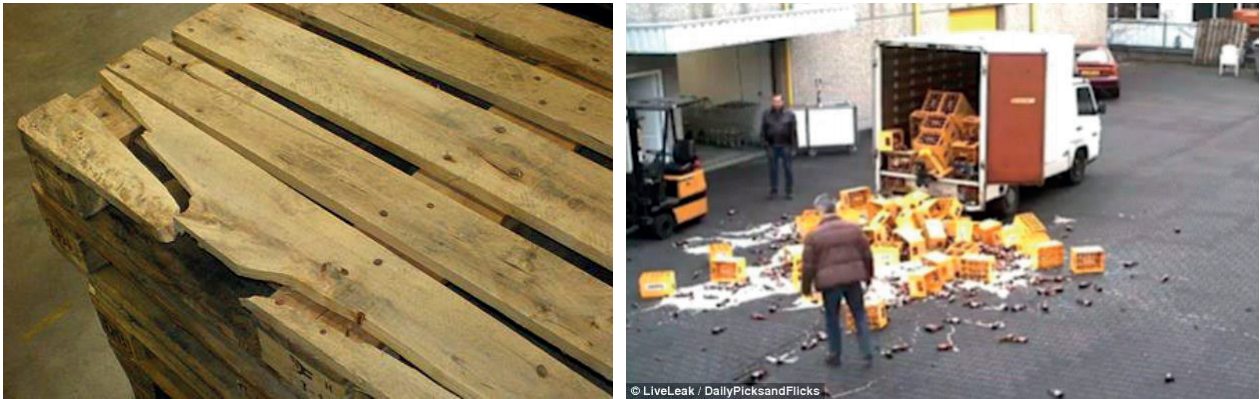
Figure 8 - Examples of breakage of a pallet top board and damage to packages of goods during vehicle unloading
