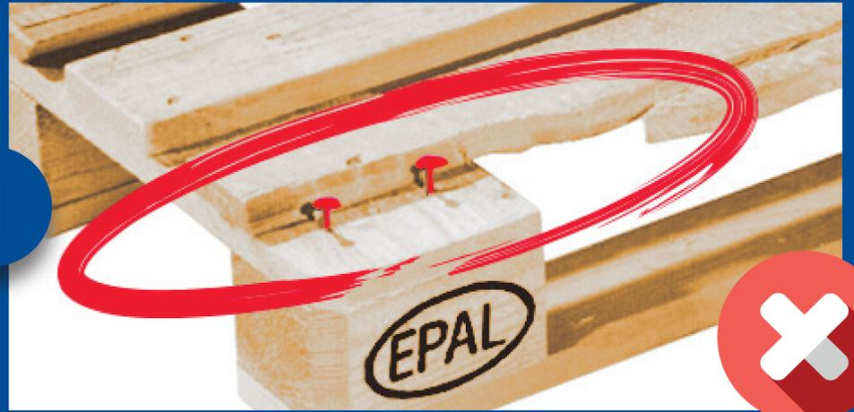
One of the deck boards is damaged, leaving nails exposed
