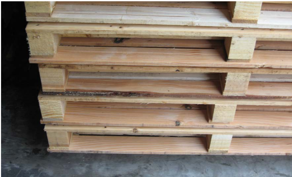
Bark on the edge of the board is less than 3 cm wide and therefore the pallet complies with bark tolerances
