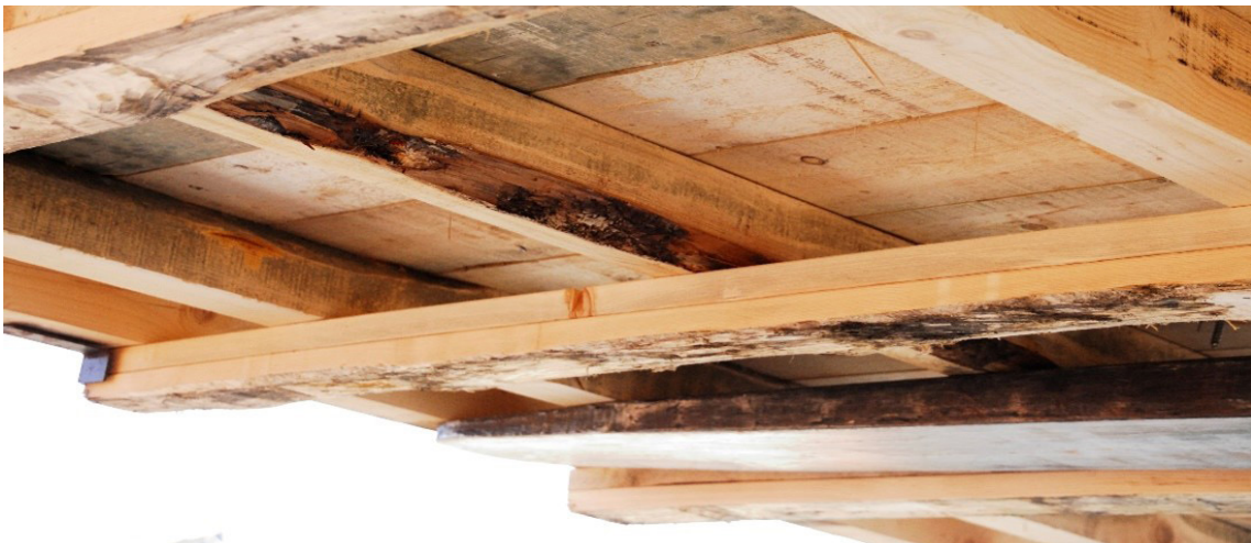
Bark exceeds tolerances: this unit of wood packaging material does not comply with ISPM 15
