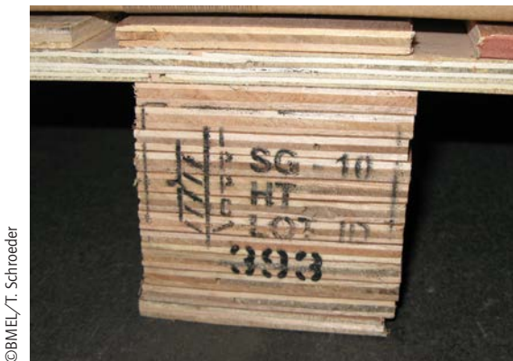
Vertical line to right of symbol is missing, additional information is included within mark, and mark is applied to processed wood
