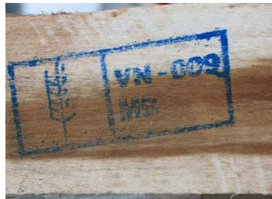
Mark, applied with an ink stamp, matches example 1 of Annex 2 of ISPM 15
