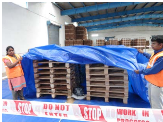
Preparing to fumigate wood pallets under gas-proof sheets or covers
