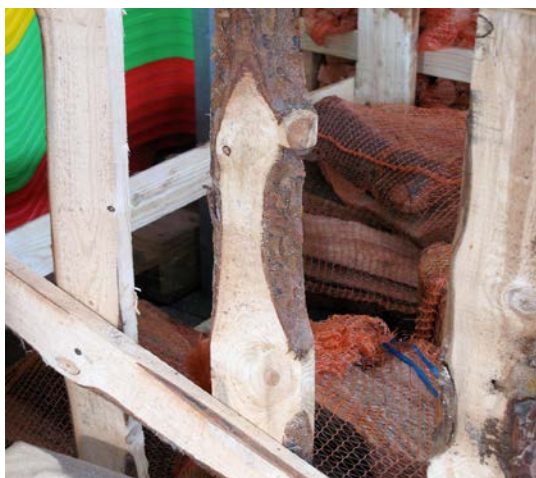
Bark exceeds tolerances: this wooden crate does not comply with ISPM 15
