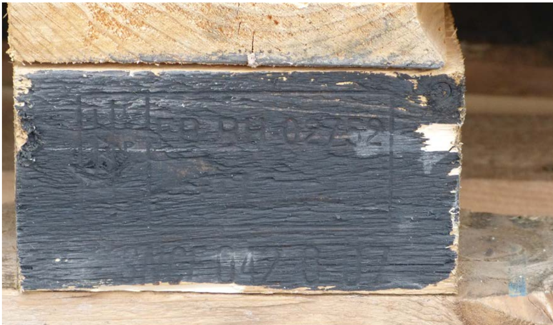
Figure 1: Example of an ISPM 15 mark obliterated with black paint
