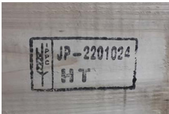
Mark, applied with an ink stamp, matches example 1 of Annex 2 of ISPM 15 but with rounded corners to the outer border as in example 3
