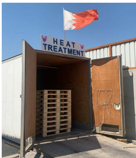
ISPM 15 heat treatment chamber in Bahrain
