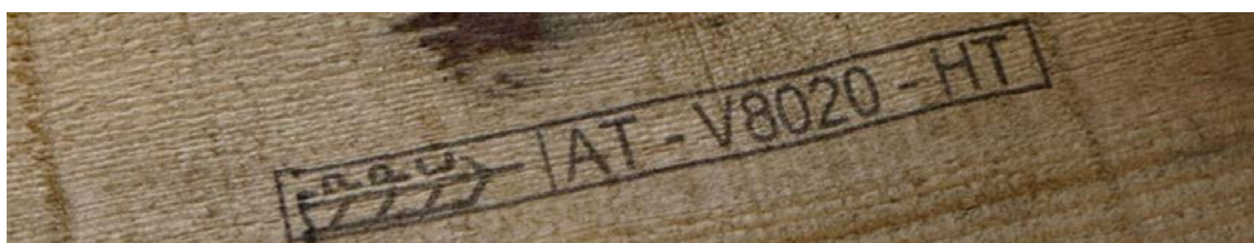
Mark with country code, producer/treatment-provider code and treatment code presented on the same line and separated by hyphens, as per example 6 of Annex 2 of ISPM 15
