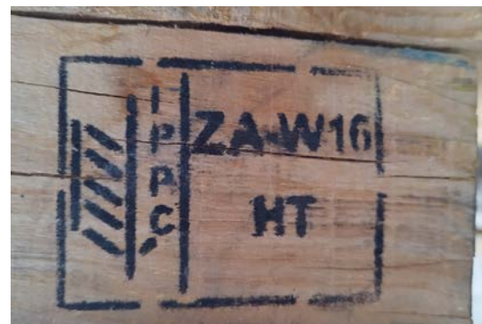
Mark, applied by stencilling, matches example 4 of Annex 2 of ISPM 15, with small gaps in the border and the vertical line
