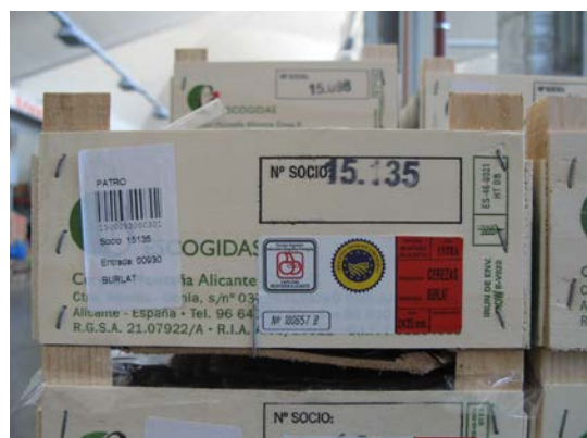
Fruit box made with solid-wood corner pieces that are larger than 6 mm
