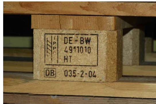
Mark, applied with a fire-brand stamp, is similar to example 2 of Annex 2 of ISPM 15 but producer/treatment-provider code is split over first and second line
