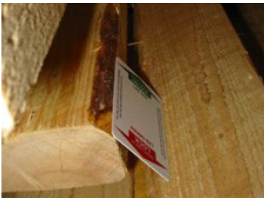
Bark on the edge of the wood is wider than 3 cm and the piece is greater than 50 cm 2 : the bark must be removed, or the piece may not be used for dunnage or to construct wood packaging material
