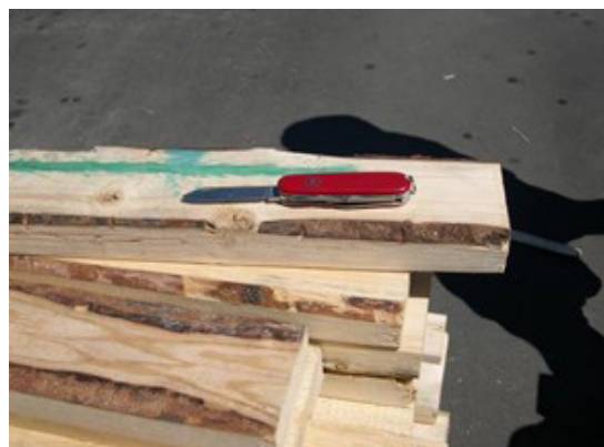
Board with knife on it is compliant because the knife is 2 cm by 15 cm and so the bark on the edge of the board is within tolerances; the board below it only contains discoloured cambium (no bark) and is therefore also compliant
