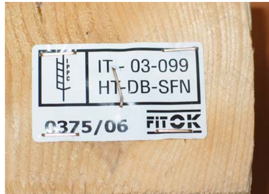
Transferable mark (mark must not be transferable; tags are non-compliant with ISPM 15)
