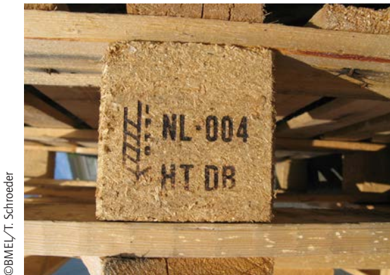
Border around mark is missing
