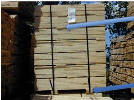
Dunnage that is integrated into packs of wood, such as the spacers or blocks indicated by arrows in this photograph, is not wood packaging material and does not need to be individually marked
