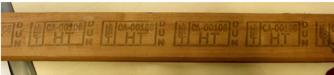
Mark matching example 1 of Annex 2 of ISPM 15 has additional information adjacent to the mark to indicate that the material is certified for use as dunnage
