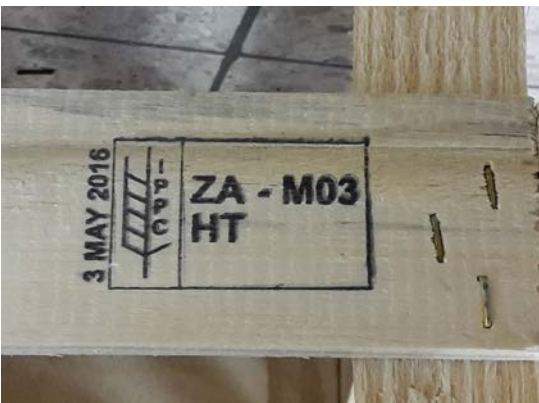
Mark, applied with an ink stamp, matches example 1 of Annex 2 of ISPM 15 and has additional information adjacent to the mark
