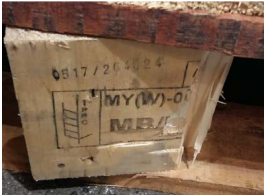
Mark is damaged and not legible
