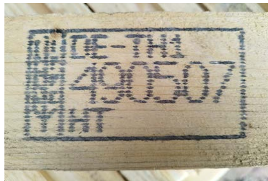
Mark, applied by an inkjet printer, is similar to example 2 of Annex 2 of ISPM 15 but producer/treatment-provider code is split over first and second line
