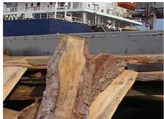
Bark exceeds tolerances: this ship-borne dunnage does not comply with ISPM 15
