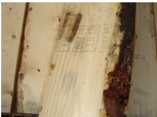
Bark on edge of board is less than 3 cm wide and therefore the board complies with bark tolerances
