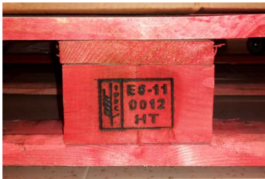
Mark, applied with a fire-brand stamp, is similar to example 2 of Annex 2 of ISPM 15 but producer/treatment-provider code is split over first and second line
