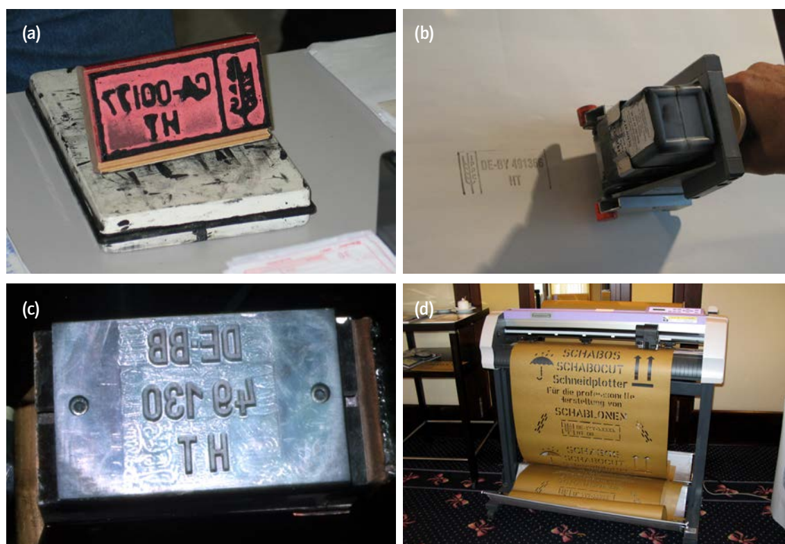
Figure 4: Examples of common methods used to apply the ISPM 15 mark
