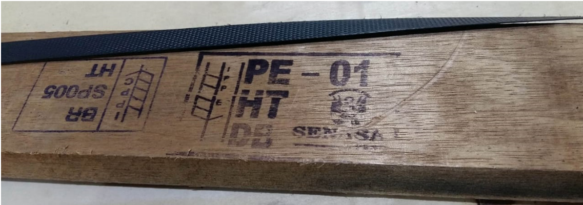
Two different ISPM 15 marks on one piece of wood packaging
