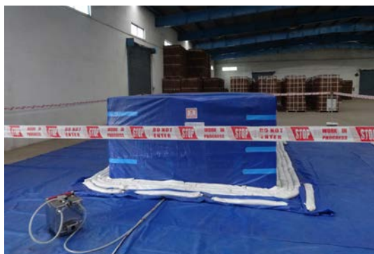
Wood pallets sealed under gas-proof sheets or covers
