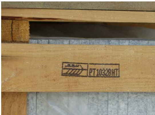
No hyphens between ISO country code, producer/treatment-provider code and treatment code
