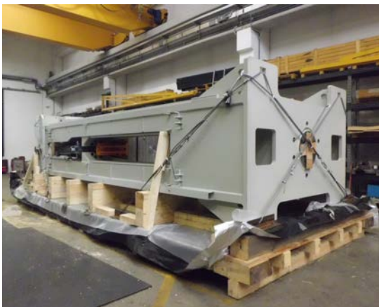
Heavy industrial wood packaging, including blocking (pieces of wood that are used to support sawn wood)
