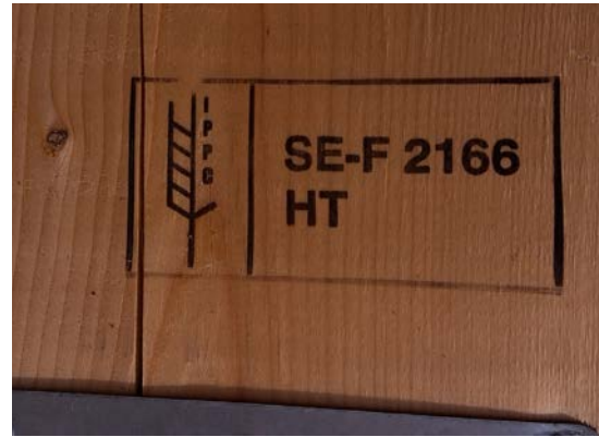
Mark, applied with a fire-brand stamp, matches example 1 of Annex 2 of ISPM 15
