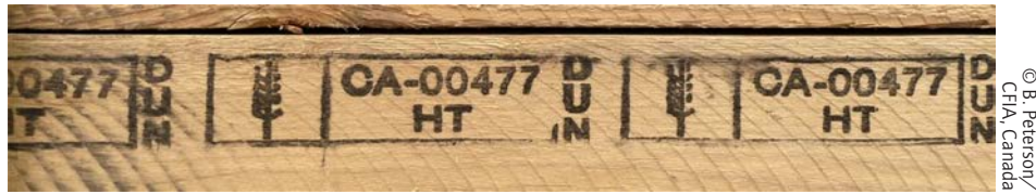
Wood packaging material bearing multiple ISPM 15 marks, for use as dunnage
