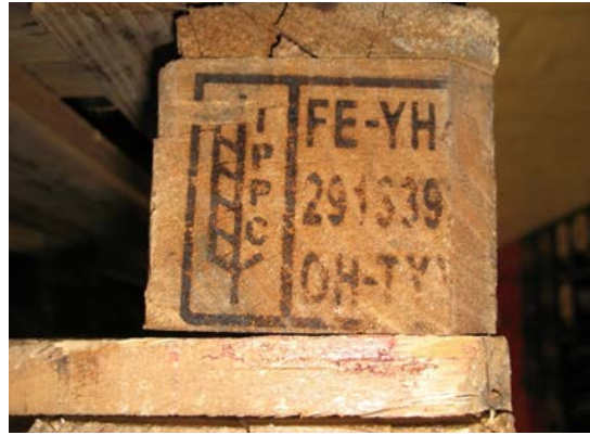
Fraudulent mark with invalid codes (no country with code "FE" and no treatment with code "OH")
