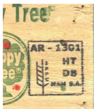
Figure 3 6 – Orientation of information does not match the examples in Annex 2 of ISPM 15:2009. Information included within the borders of the mark exceeds the requirements.
