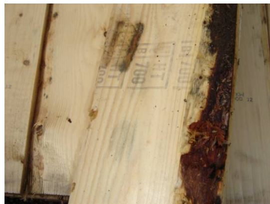
Figure 2 - Bark on edge of board is less than 3 cm wide therefore the board complies with bark tolerances.
