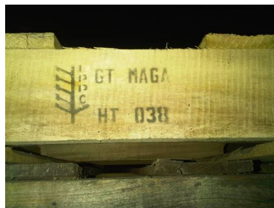
Figure 4 6 – Mark does not contain the required borders.
