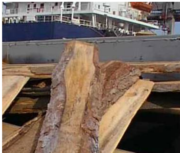
Figure 6 - Bark exceeds tolerances. This ship borne dunnage does not comply.
