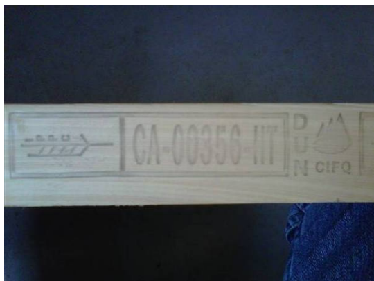
Figure 1 5 – Mark matches example 6 of Annex 2 of ISPM 15:2009. Additional information included outside the borders of the mark.
