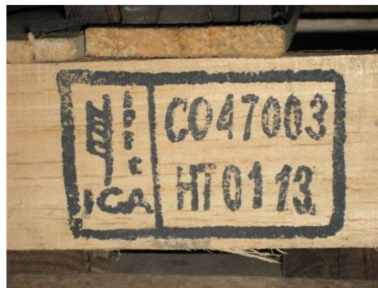
Figure 2 6 – Information beyond what is prescribed in Annex 2 of ISPM 15:2009 contained within the borders of the mark.
