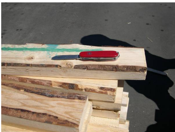
Figure 3 - Bark on the edge of the board. The knife is 2 cm by 15 cm, therefore the board complies with tolerances. The board below the one with a knife, only contains wane (discoloured cambium) and is therefore compliant.
